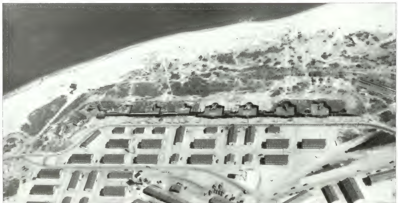
Figure 5.20. Oblique aerial view of Nine Gun Battery, 1942. This World War II-era photograph of Nine Gun Battery, and a portion of Battery Peck (left), indicate they were both finished with an asphalt emulsion paint (also refer to cover photograph). This surface treatment has worn away from gun platforms #3 and #4 (center) and the brighter appearance of the concrete underneath is visible (National Archives, Record Group 661 S, Philip S. Gage Collection, Fort Hancock Folder).
